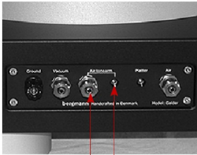
Pic. 16. adjustment valve for airbearing tonearm air out put for airbearing tonearm
