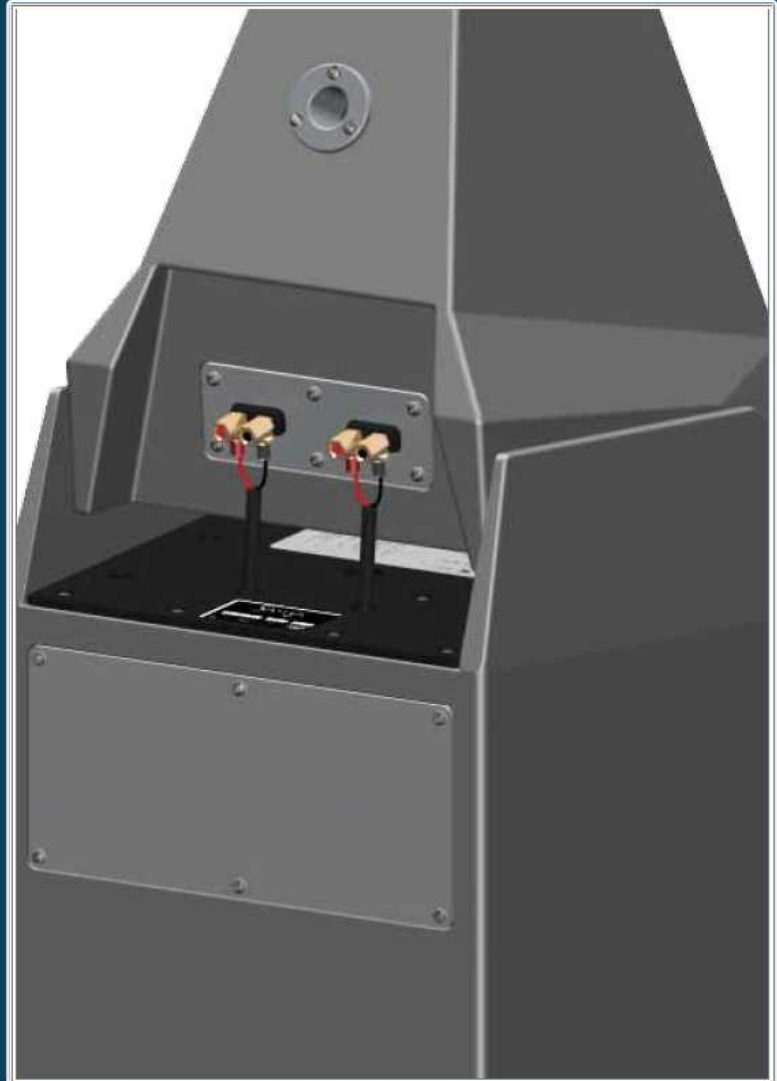
FIGURE 6 – CONNECT THE UMBILICALS TO THE TWO UPPER MIDRANGE/TWEETER MODULE INPUTS, OBSERVING CORRECT POLARITY.
